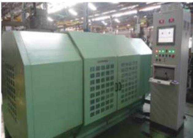
Vibration of an electrical motor is closely related to its assembly With the driven equipment. To evaluate the vibration levels of motor alone, it is necessary to measure the same in uncoupled and free shaft condition with a half key fitted in key way on shaft and in freely suspended state with the help of a string as specified in IEC60034-14. The motor is said to have vibration if any part of it experiences displacement / velocity in any direction beyond the limits specified in the table 4.
