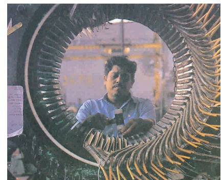
Fig. 2 Coil Setting thermosetting varnish and baked – the number of dipping and baking cycles depending on the type of environment and service condition.
